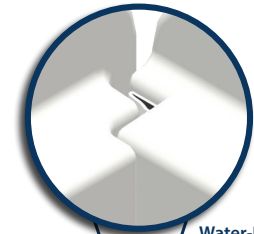
Water-Proof Gasket (Magnified View)
